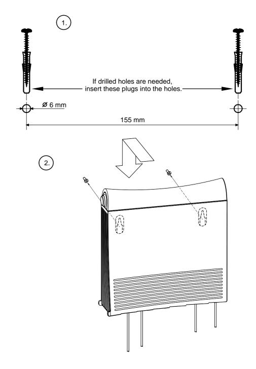
Figure 6. Wall installation
